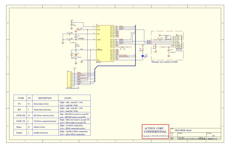
PCB footprint & dimensions, part number, supplier and pinout spec for the connector J1 on ACT-IR8250x0PMB and ACT-IR8250PDB boards are as follows: Molex, part number SD-48148. You can get dimensional information at: <u>www.molex.com</u>. More details on <u>section 5.1</u>.
