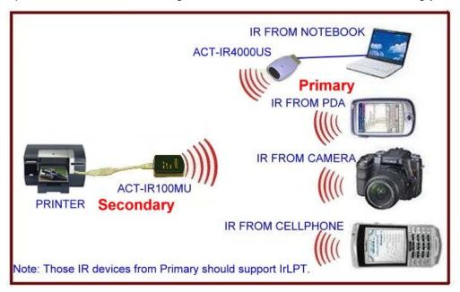
Figure 1: SYSTEM DIAGRAM FOR ACT-IR100MU
