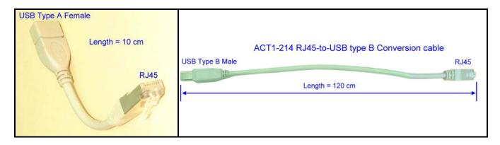
Fig. (L): RJ45-USB type A Cable; Fig. (R): ACT1-214 RJ45-to-USB type B direct conversion Cable
