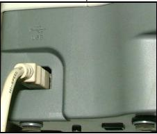
**Step3:** Connect RJ45-USB conversion cable (This cable is only for converting RJ45 to USB interface) to ACT-IR100MU as shown at below point A.
