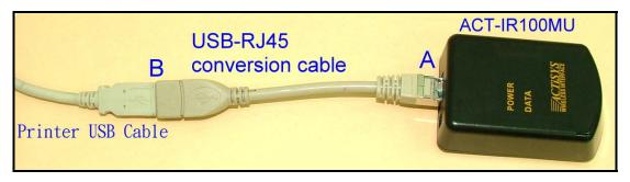
**Step4:** Connect printer USB cable from printer to USB-RJ45 conversion cable as shown at above point B
