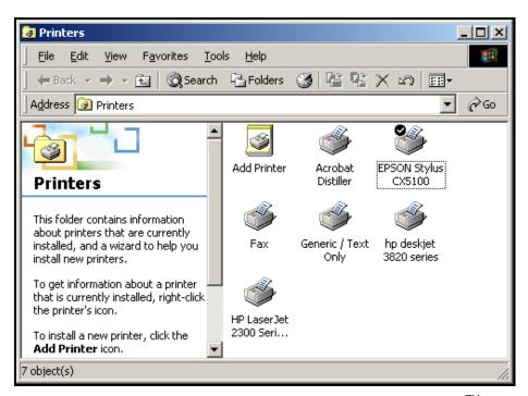
**Step8:** Assign IR port to your printer driver. This builds up IrLPT<sup>TM</sup> structure for your sender.
