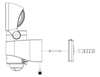
Be careful not to damage the mounting bracket as it also serves as the back of the light and the battery cover.
