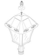
7. Assemble pole (J) by screwing the four pieces together.
