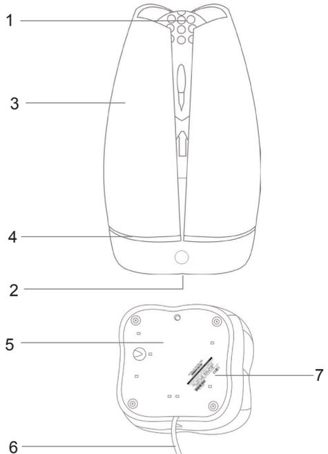
It is possible to adjust the light intensity/color using the night light intensity touch sensor (2) located at the position indicated by the illustration above. The light does not intervene or has any relation with Airfree's TSS™ patented sterilization core functioning.
