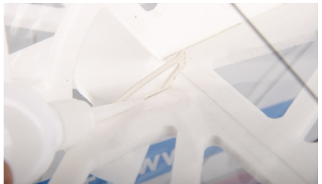
25. Install elevator control horns.
