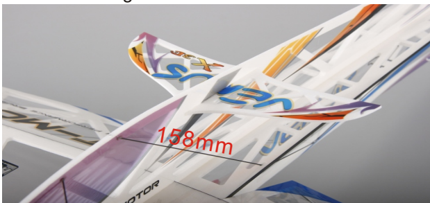
22. Install 2pcs carbon fiber rods between upper horizontal fuselage and vertical fuselage. Refer to picture.
