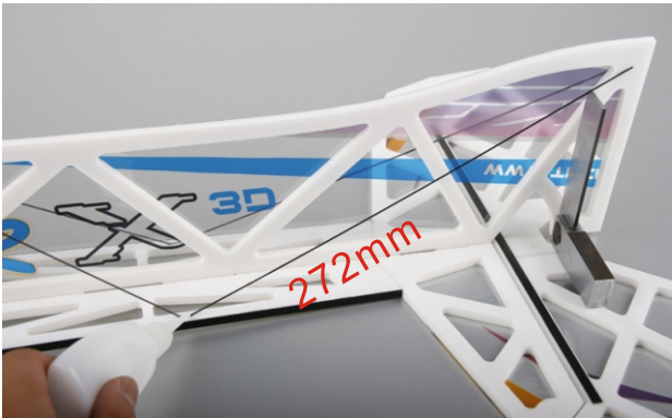
13. Fix landing gear reinforcements to corresponding hole with glue.
