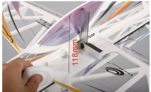
18. To avoid distortion on vertical fuselage, install 2pcs carbon fiber rods between upper horizontal fuselage and vertical fuselage.
