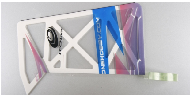
16. Insert upper vertical fuselage into the slot of horizontal fuselage, then use CA to fix. Notice: make sure both fuselages are perpendicular to each other.
