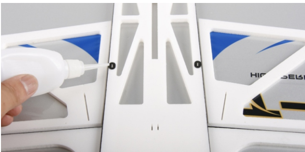
8. Insert above carbon strip into pre-reserved slot on bottom vertical fuselage (close to the nose), then fix with glue. Make sure the 9-hole reinforcement is perpendicular to vertical fuselage.
