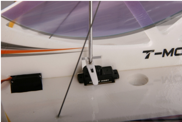
32. Install rudder servo arm extension.
