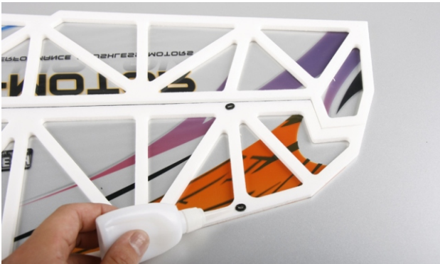
7. Glue 9-hole carbon fiber reinforcement and 1pc 3*10*1mm carbon fiber strip together.
