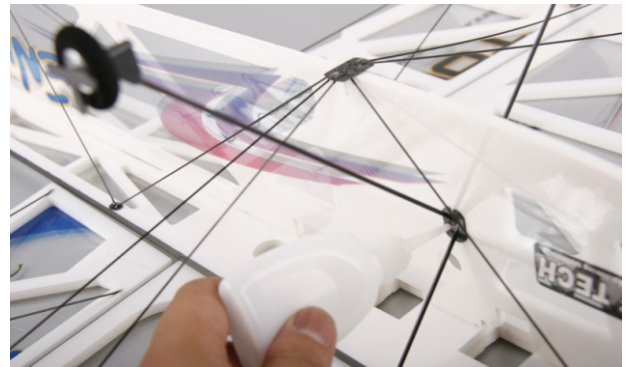
13. Fix landing gear reinforcements to corresponding hole with glue.
