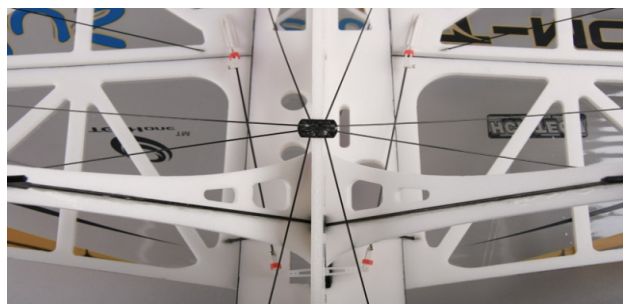
31. Install aileron push rods. Make sure the both aileron control surface is at the same angle.
