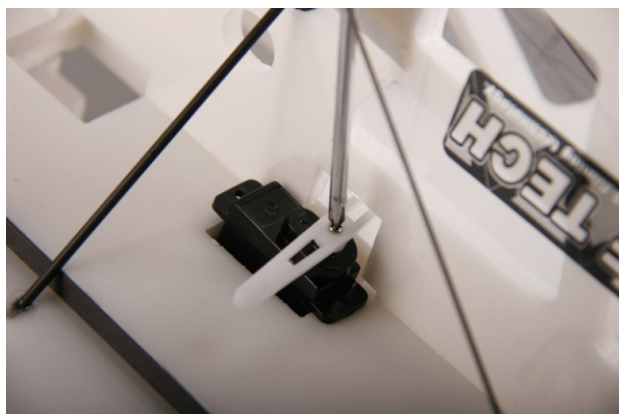
29. Use screwdriver to install aileron servo arm.
