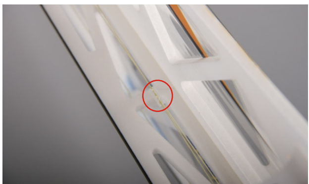
39. Install elevator pull-pull thread. Same operation as rudder pull-pull thread.
