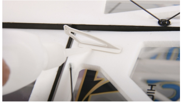
23. Install aileron control horns on back wings.
