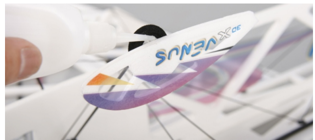
14. Install landing gear sets.
