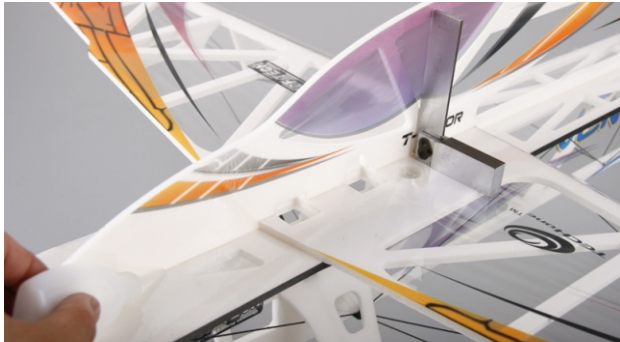
16. Insert upper vertical fuselage into the slot of horizontal fuselage, then use CA to fix. Notice: make sure both fuselages are perpendicular to each other.
