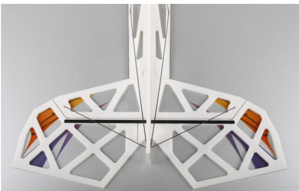
12. Install other carbon rods, and make sure the vertical fuselage is perpendicular to wing.
