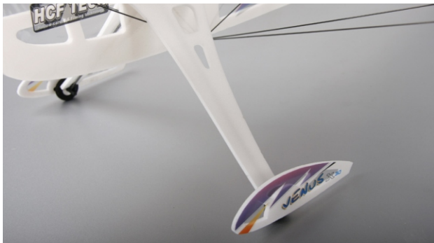
15. Install wheel covers and landing gear baffle.
