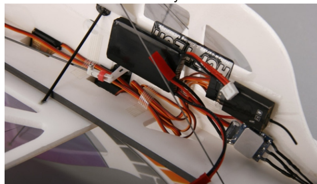
43. Pass all servo wires through fuselage and place them close to receiver.
