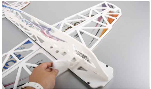
6. Insert vertical fuselage into the slot of horizontal fuselage, then use CA to fix. Notice: make sure both fuselages are perpendicular to each other.
