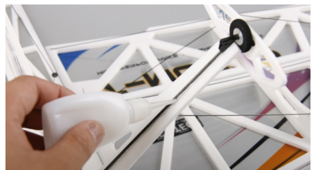
12. Install other carbon rods, and make sure the vertical fuselage is perpendicular to wing.
