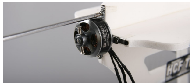
26. Install motor on motor mount with 4pcs self tapping screws.
