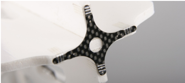
20. Install motor mount on nose, then use fiber tape to reinforce.
