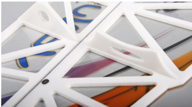
9. Install wing fences on corresponding places of bottom wing and fix with glue.
