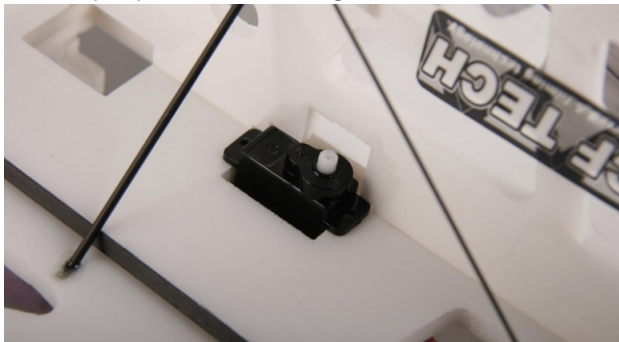
28. Place aileron servo into pre-cut servo hole on fuselage and fix with glue.
