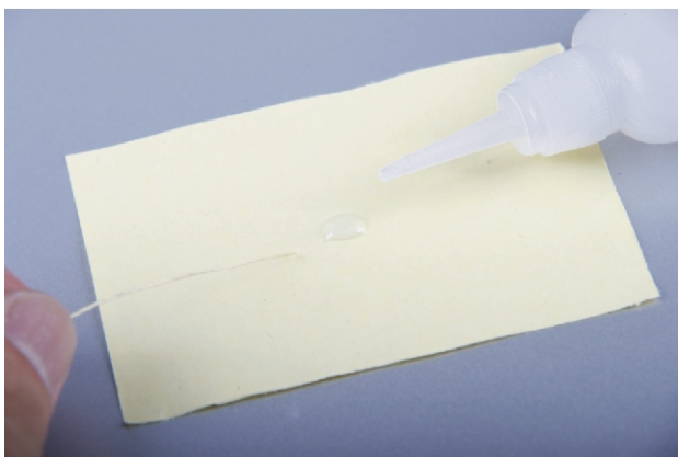
33. Drop some CA on the ends of thread to make them a little harder, so they can easily thread through small holes.
