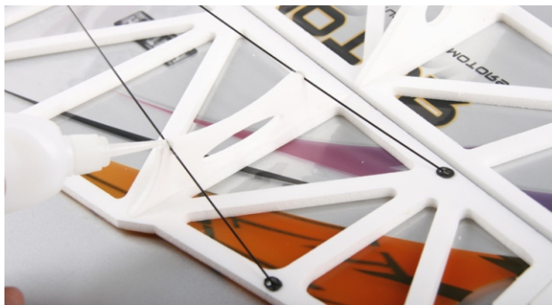
9. Install wing fences on corresponding places of bottom wing and fix with glue.
