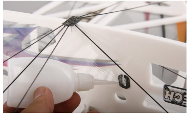
13. Fix landing gear reinforcements to corresponding hole with glue.
