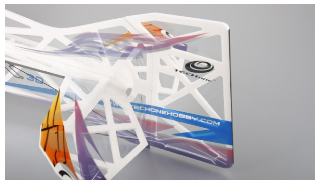
17. Install rudder on vertical fuselage.
