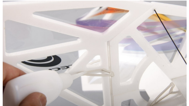
24. Install rudder control horns.
