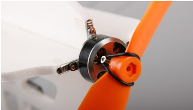
27. Fix propeller with o ring.
