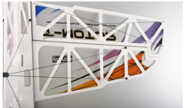
11. Install aileron carbon fiber rods, no distortion on ailerons.
