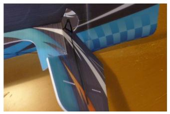
Insert the 0.5 mm x 32.5 cm carbon strip in the elevator control horn. Then glue them together in the pre-reserved slot. ATTENTION: elevator and rudder control horns are asymmetric. The shorter part goes on the side of mobile surface where there is the bevel for movement.
