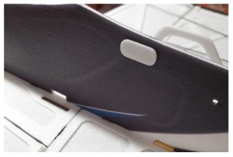
Fix with C/A the two 2 mm depron reinforcement parts on both sides of lower vertical fuselage. A micro hole indicates the position. In a consecutive step you will have to insert in it the four 1.5 mm carbon rods to reinforce the wings.
