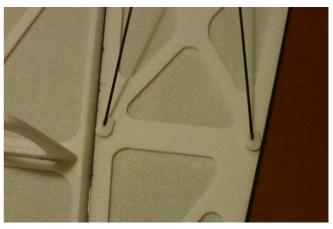
Fix with C/A the four 2 mm depron reinforcement parts on the bottom of wing at the end of each 1.5 mm wing carbon rod.
