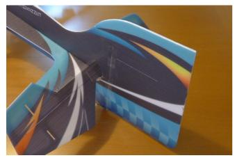
Install the rudder to the fuselage with some 3M tape.
