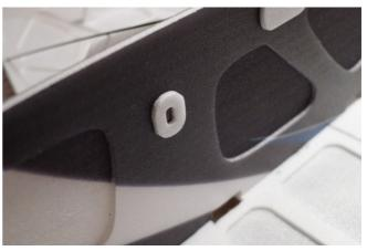
Fix with C/A the two 2 mm depron reinforcement parts on both sides of lower vertical fuselage where there is the hole for the landing gear legs.
