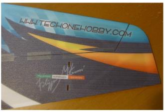
Fix the elevator with 3M tape.Do the same with ailerons.
