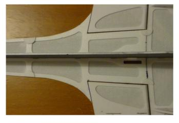
Fix with C/A the four 2 mm depron reinforcement half-moons on the bottom of horizontal fuselage as shown in the picture. The micro holes indicate the position. They are necessary to reinforce the points where the 1 mm carbon rods will be fixed.
