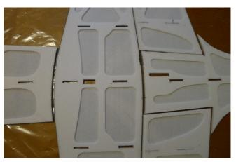
Fix the horizontal fuselages to the wing with  $\mathbf{C}/\mathbf{A}$ .
