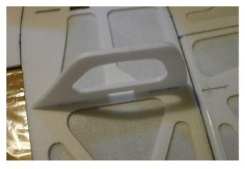
Insert the downside vertical winglets into the pre-reserved slots on the downside of the wing and apply some C/A to fix.
