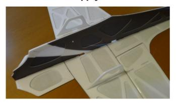
Use some C/A to fix the lower vertical fuselage on the horizontal fuselage. Be vertical and no distortion!
