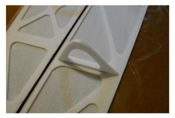
Insert the parts to reinforce control surfaces into the pre-reserved slots on ailerons and apply some C/A to fix.
