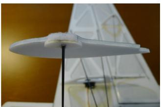
Fix the small depron piece to the wheel pants to reinforce them. Pierce the wheel pants and fix them with C/A in the landing gear as shown in the picture. Fix with C/A a small piece of velcro on each wheel pant.
