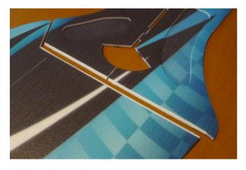
Cut a 55° bevel on ailerons. On elevator and rudder cut a 40° bevel on mobile and fixed surface.
