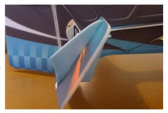
Insert the four 2 mm winglets into the pre-reserved slots on the elevator and apply some C/A to fix.
