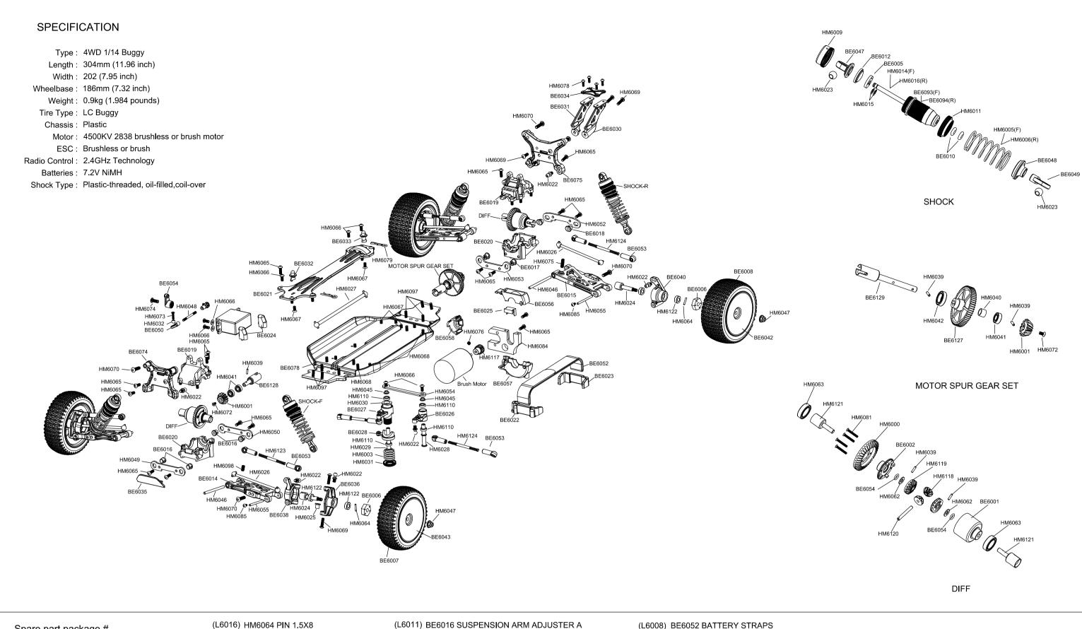
(L6023) HM6045 STEERING LINK BUSHING (L6006) HM6046 HINGE PIN (L6041) HM6047 M3 FLANGE LOCK NUT (L6024) HM6048 SERVO CONNECTING LINK (L6011) HM6049 SUSPENSION MOUNT FF (L6011) HM6050 SUSPENSION MOUNT FR (L6011) HM6052 SUSPENSION MOUNT RR (L6011) HM6053 SUSPENSION MOUNT RF (L6023) HM6054 STEERING PLATE (L6006) HM6055 LOWER ARM SHAFT (L6015) HM6062 WASHER 3X6X0.5 (L6042) HM6063 BEARING 8X12X3.5
