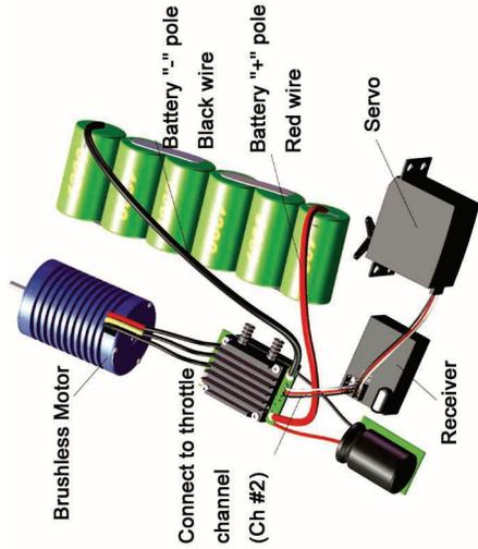
**STEP #2. Throttle Range Setting (Throttle Range Calibration)**
