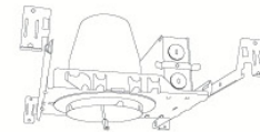
4" Standard ICA Housing 750 lm (11.8W) w/ELK19 Series Module 950 lm (11.8W) w/ELK21 Series Module New Construction
