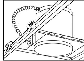
**Step 1.** Locate center of proposed opening on ceiling tile and cut appropriate sized hole.\*
