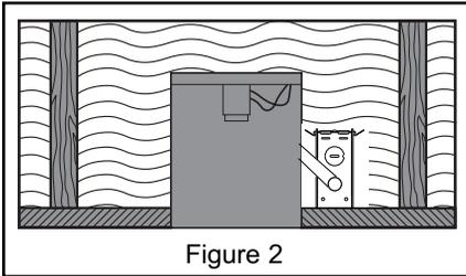
Juno Type IC fixtures are designed for direct contact with insulating materials which are approved for this application (Fig. 2). Blinking light after installation indicates that improper bulb or trim is being used.
