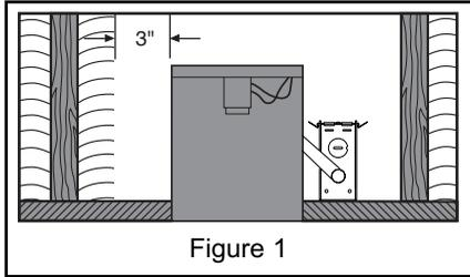
Juno Type TC & PL fixtures are designed for installations where housing and J-Box will not come into contact with insulation. Insulation must be spaced 3" away from the housing and J-Box (Fig. 1)\*. Blinking light after installation indicates that improper bulb or trim is being used or that fixture has been improperly covered with insulation.
