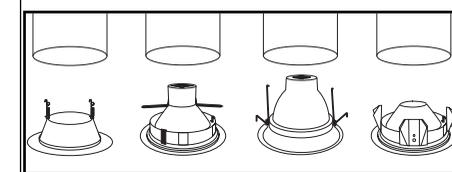
Install trim using coil, leaf, torsion, or push-in springs as provided. Remove socket paint protector cover and install proper lamp as listed on housing label.
