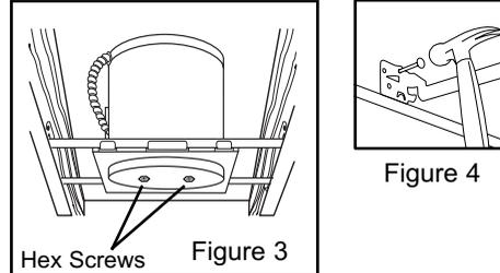
**Step 1.** Extend bar hangers to fit between joists. Bar hanger foot is contoured to easily align with bottom of joist (Fig. 3). Position fixture by hammering Real-Nails™ into joists (Fig. 4).
