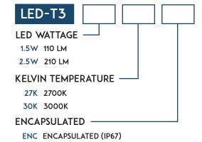
+ Dimmable: See ENCAPSULATED T3 LED Lamps Spec Sheet for additional details
