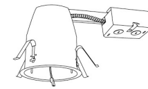
3" ICA Housing Remodel
