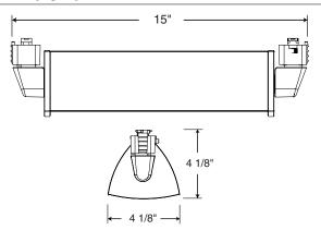
Alternate TEK/HTEK Trac Adapter Compatible with either Juno TEK or HTEK trac systems • System specific and assembled to trac fixture • Integrally polarized construction to prevent reverse installation - only allows insertion in proper orientation • Rotary circuit selector enables simple switching between circuits • Integral on/off switch enables individual fixtures to be switched for servicing.
