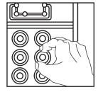
Next, plug in and turn ON the lamp or radio at the receptacle's other outlet to make sure the power is OFF at both outlets. If the power is not OFF, stop work and call an electrician to complete the installation.
