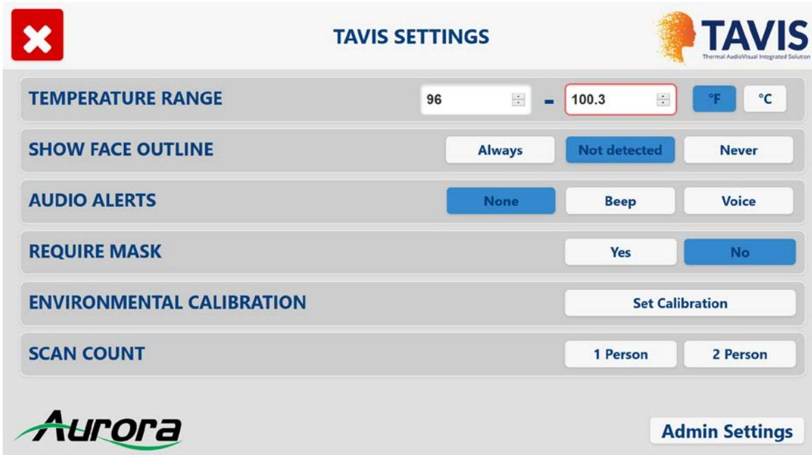
**TEMPERATURE RANGE:** This setting will determine the minimum and maximum temperature allowed before raising a flag that the person being scanned has an elevated skin temperature. The audio alert will play through the tablet’s speakers when the sensor records a temperature higher than the maximum temperature. You may display your temperature in Fahrenheit or Celsius by selecting °F or °C.
