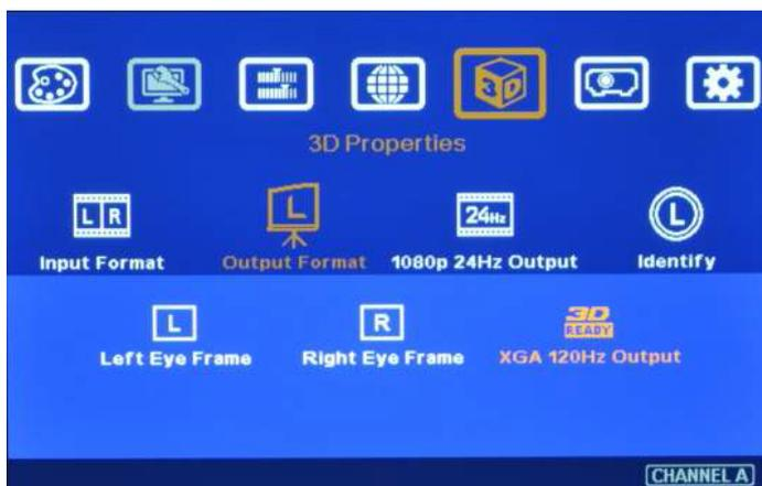
3. If user selects other output resolution except XGA or 720P, [3D Ready] menu will be grayed out and user can't select 120Hz output.
