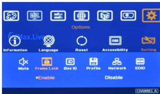
[Frame Lock] will ensure the input and output frame rate synchronize together.
