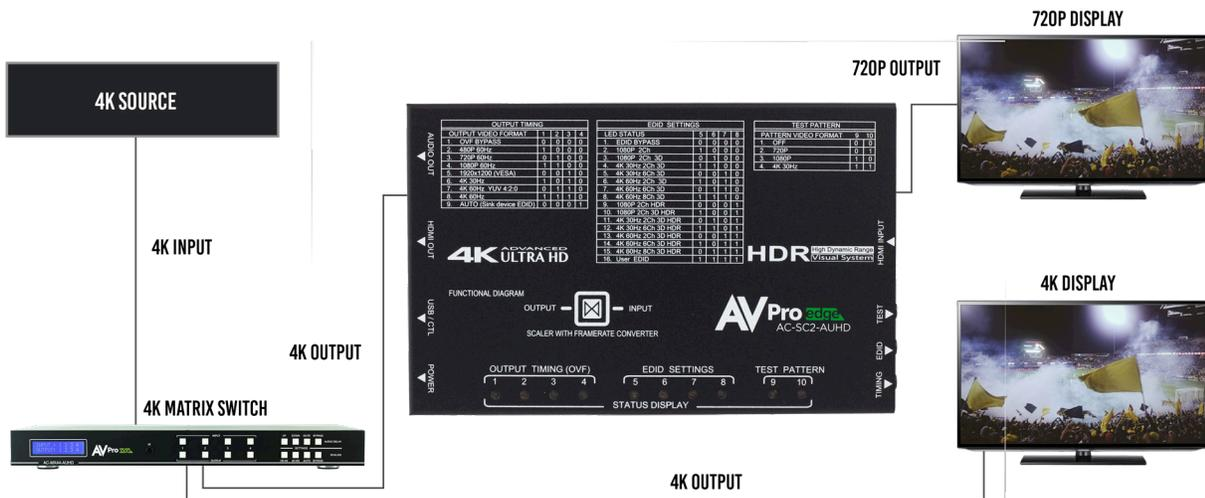
WITH THE AC-SC2-AUHD YOU ARE ABLE TO DOWNSCALE (AS SHOWN) OR UPSCALE A SIGNAL TO DISTRIBUTE THE BEST POSSIBLE PICTURE TO ANY DISPLAY.
