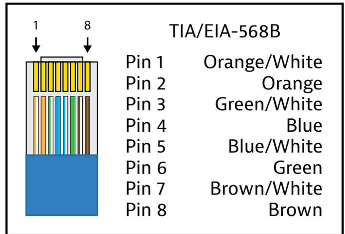
**Twisted Pair Wiring:** Use the TIA/EIA-568B wiring pattern when making RJ45 connections between the host and client extenders.
