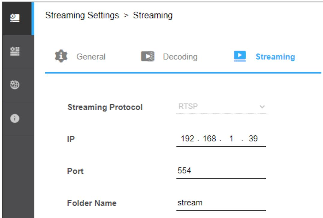
Figure 13: Streaming Settings – Decoder Streaming Tab
