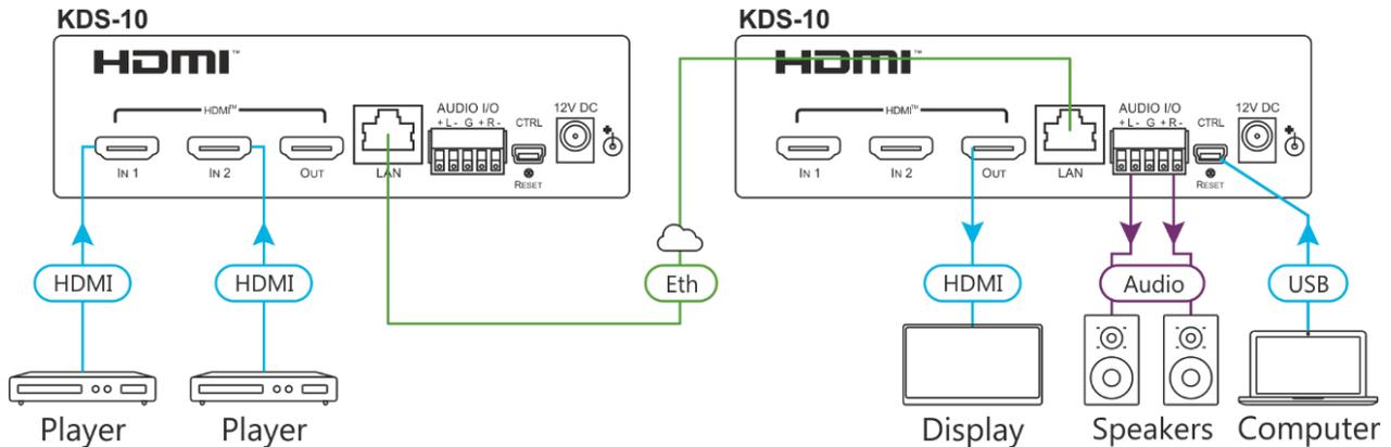
Figure 2: Connecting to the KDS-10 Rear Panel
