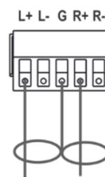
Figure 4: Connecting to an Unbalanced Stereo Audio Acceptor
