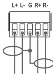
Figure 3: Connecting to a Balanced Stereo Audio Acceptor
