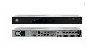
KN-100 is server hardware with Kramer Network software already installed on the device. With a 6th generation Intel® Xeon® E3-1240 v5 Xeon (4 Cores, 8M Cache, 3.50 GHz) processor, 2x 4GB DDR4 RAM, an 80GB SSD hard drive, Windows® 10 operating system, KN-100 is designed to maximize the features and benefits of Kramer Network.
