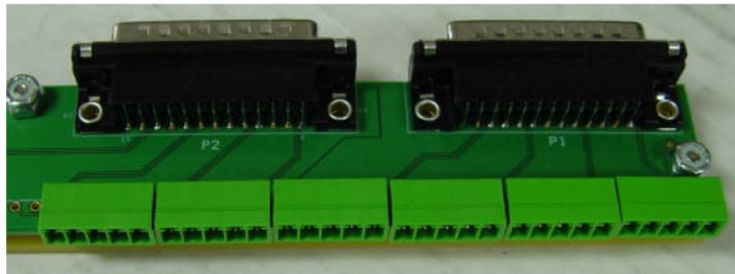
The 25-pin “D” connectors each support a group of 4 inputs or outputs and the screw terminals are in groups of 4 containing 2 inputs or outputs each.
