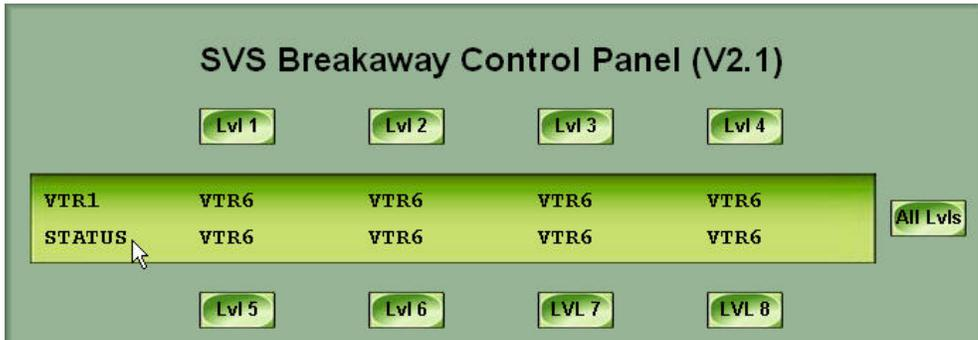
**“Programmable Control Panel”** adds 8x8 programmable XY buttons for single-button takes.
