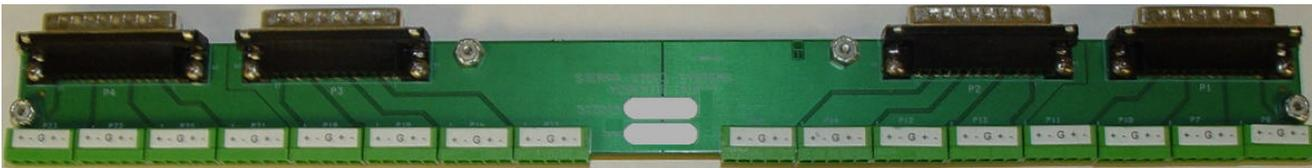
Each adapter panel connects to 4 of the 25-pin “D” connectors. This connects a total of 32 inputs or outputs.
