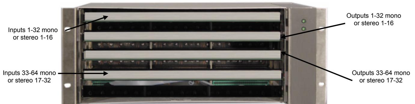
The top slot in both the analog and digital frame contains the input buffer module for inputs 1-32.
