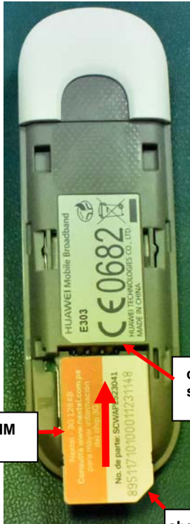
3- Set SIM card on modem below card slot. The chamfered corner is at bottom right.
