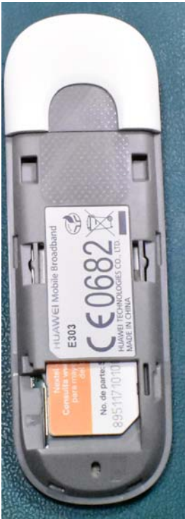
4- Slide SIM card into slot fully. (Card is fully in slot above)
