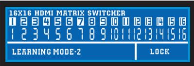
4. Press **ENTER** to confirm changes. The LCM will return to the default screen selected switch routing status.
