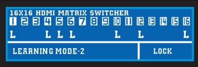
3. Press **DESTINATION 1 THRU 16**. The switcher will LEARN destination HDMI EDID and pass to the selected source. The switcher will Enable or Disable HDMI EDID for the selected source.
