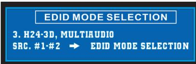
Select & change current EDID mode via (7) Embedded EDID modes. Used to display and change current EDID mode.
