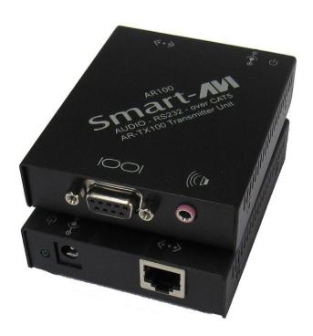
The AR100 RS232 - Sound Cat5 extender allows you to extend any full Duplex RS232 with any Stereo sound up to 3000ft using a single unshielded Cat5 cable.
