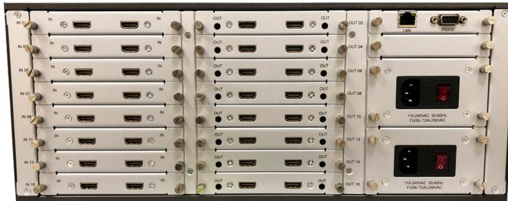
The top power-plug is 230V and is intended for use within the EU or countries where 230V is the standard. Please check all voltages and inputs before proceeding with powering on the unit.
