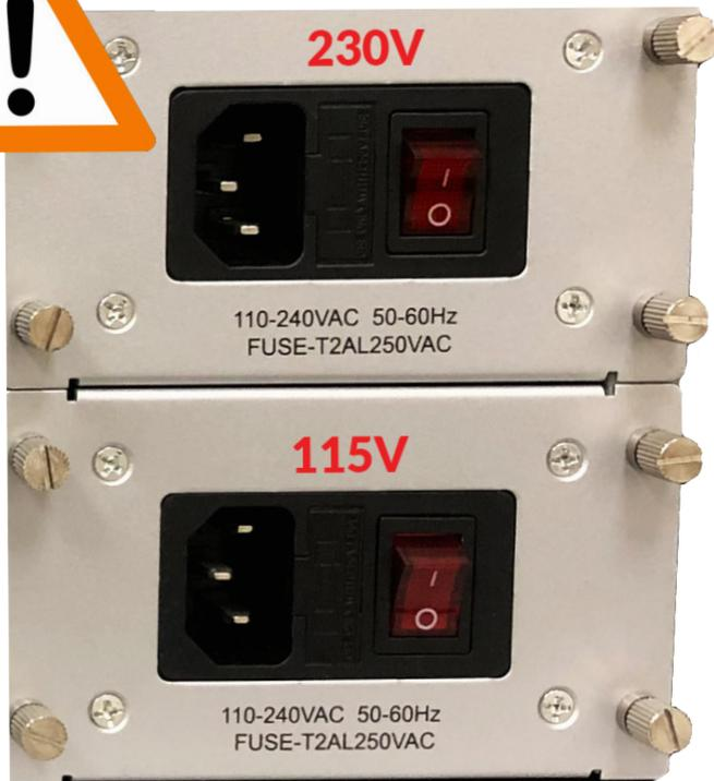
The top power-plug is 230V and is intended for use within the EU or countries where 230V is the standard. Please check all voltages and inputs before proceeding with powering on the unit.
