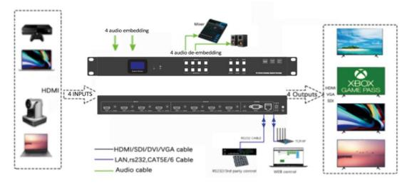
Working as 4 inputs and a 2x2 TV Wall controller:
