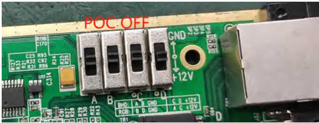
POC function OFF: Have the 4-pin DIP switch set to the middle position
