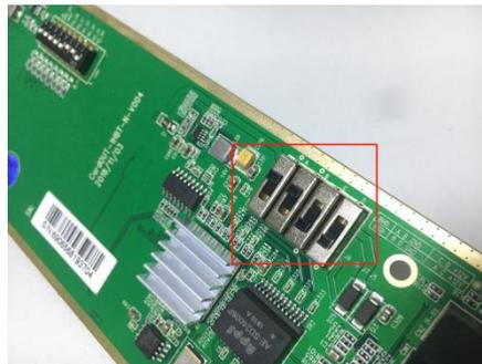
Step3: Pull all this 4-pin DIP switch to the middle position(Turn off the POC function)
