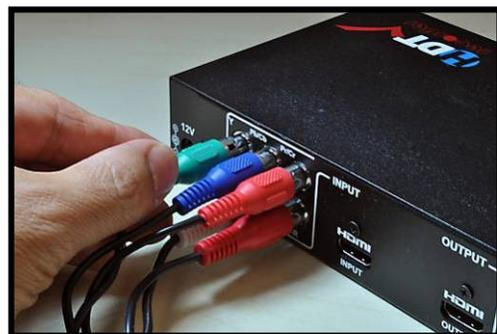
Since YPbPr video cables do not carry audio, you must also attach an audio cable between the player and recorder (bottom row); this cable will have 2 connectors (left-right speakers, usually red and white). You will need to connect a total of 5 connectors. Attach the other ends to your Video Player.
