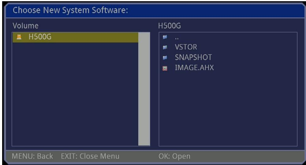
9. Search for the firmware file (file extension is .AHX) on the USB drive; arrow down to the file and press the
