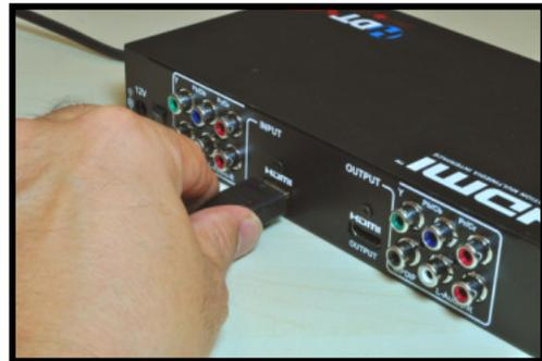
b) **YPbPr**– Connect the YPbPr cables, matching the colors between the connectors and adapters (top row - shown right). There are two audio connectors for the L-R audio connectors below the YPbPr adapters. Attach the other ends of all the cables to your HDTV.
