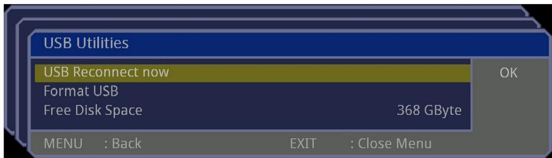
The “Format USB” item can be used to format a USB HDD, a USB Pen drive or a memory card used with a USB card reader. The HDTV Recorder formats using the FAT/FAT32 file system format. (HDTV Recorder does NOT support other file systems).
