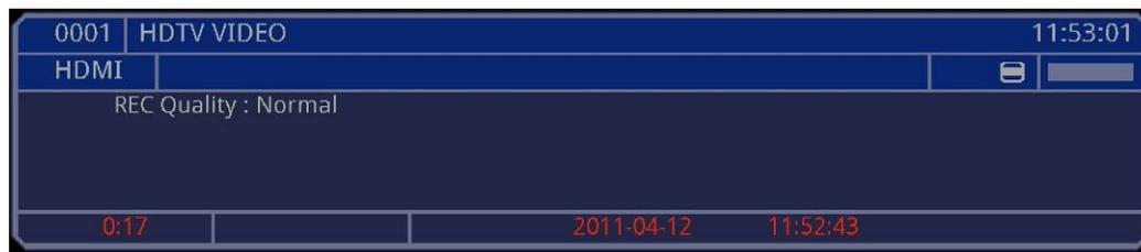
The top-right corner displays the current time and the left column (second line) shows the current input source (e.g. HDMI). The middle row shows the recording quality or compression video bit rate. The bottom line is described as follows (from left to right):
