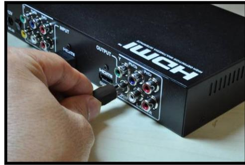
**Note:** The connections you use between input and output do not have to be the same. In other words, if you are using an HDMI cable for input, you can use YPbPr for output.
