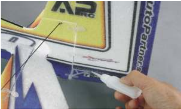
Glue the unidirectional control horn to left side of the rudder.
