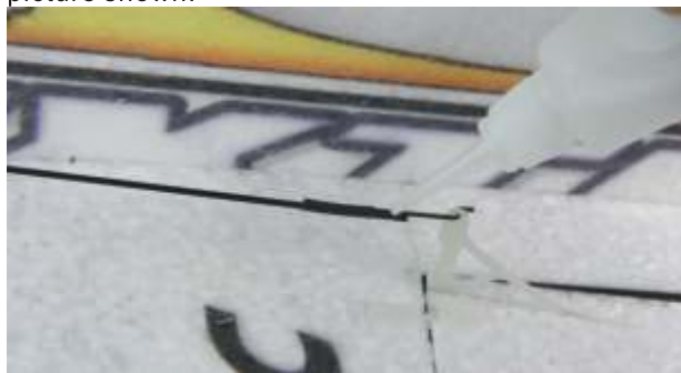
Fix the Z bend and pull-push rod with glue.
