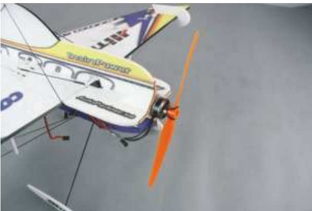
Fix propeller with o ring.
