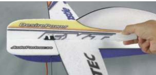
Insert the upper half part of the fuselage to the square hole of the horizontal fuselage. And then adjust it and fix with glue.
