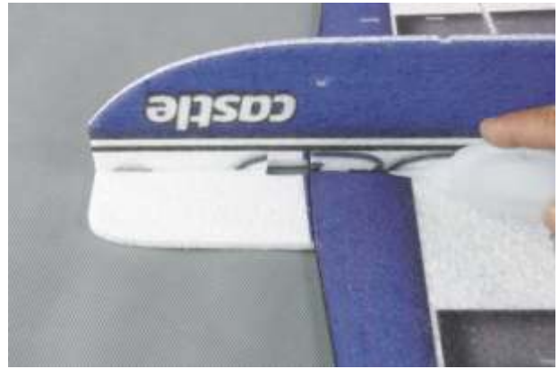
Adjust the fuselage, ensure it flat and straight, then fix it with glue.
