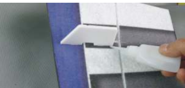
Insert the support board of the wing to the pre-reserved square holes, and fix it with glue.
