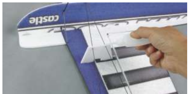
First fix the left and right support rods with glue as picture shown.
