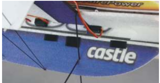
Cut off three pieces of velcro, they are used for installing receiver, ESC and battery.
