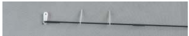
Thread 2pcs support rods and 1pc shrink tube through the elevator pushrod, then connect one side with Z bend to the unidirectional servo arm.
