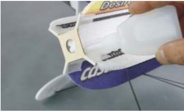
Fix the motor mount to the nose with glue.
