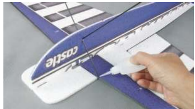
Make the 2*260mm carbon rod pass through the pre-reserved hole on fuselage, and insert it to the holes on the wing, and then fix it with glue.
