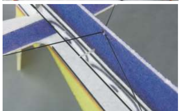
Find the right position for inserting the support rods. Please not do glue them at this step.
