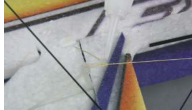
Make one of the thread end pass through the small hole on elevator, then tie a knot and glue it.
