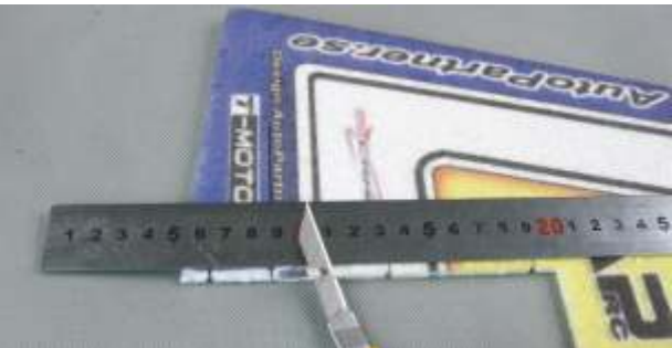
Cut off 45 bevel angle at the hinge parts.
