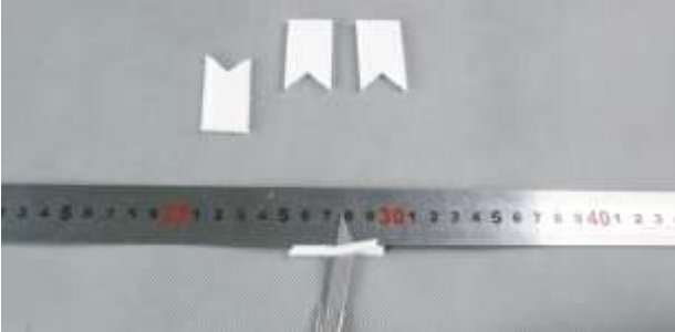
Cut off 45 bevel angle on the 4 reinforcing boards as picture shown.
