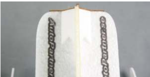
Install the reinforcing board to the nose and fix it to the motor mount with glue.
