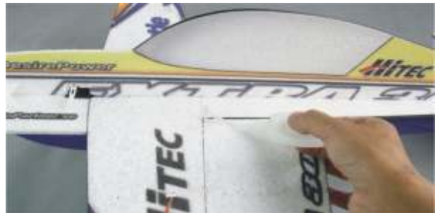
Install the control horns to the face of left and right aileron and fix them with glue.
