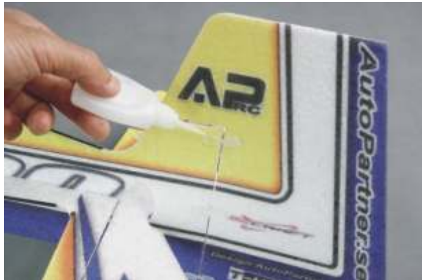
Glue the rudder and fuselage well.
