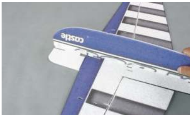
Insert the lower half part of the fuselage to the square hole of the horizontal fuselage and the wing.
