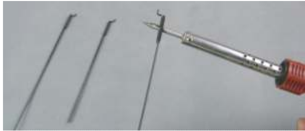
Put the shrink tubes to the pull-push rod as picture shown, and then fix it with iron heating.
