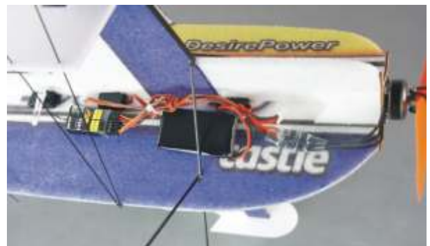
Connect well the servos and receiver. Then install the battery, ESC and receiver to the right position on nose.
