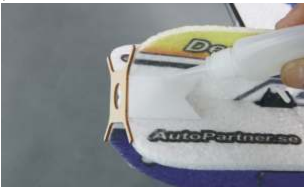
Cut off 45 bevel angle on the 4 reinforcing boards as picture shown.
