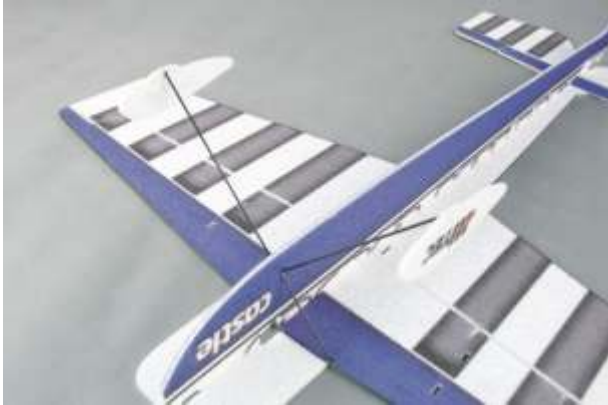
Glue the wheel cover and the carbon rods tightly.
