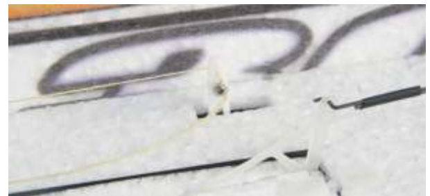
Make the other end of thread pass through the two holes on servo arm, thus the pull-push thread could not be loosed easily. Use the same way to install the other pull-push thread.
