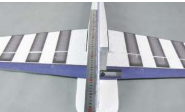
Insert the lower half part of the fuselage to the square hole of the horizontal fuselage and the wing.
