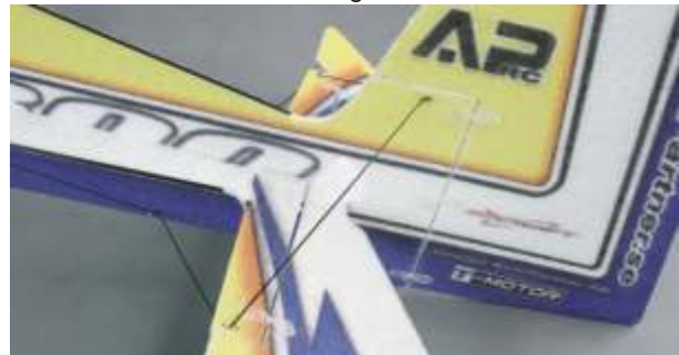
Use 1mm carbon rod to reinforce the vertical tail.
