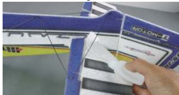
Glue the bidirectional control horn to the elevator.
