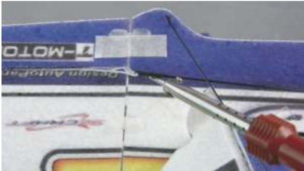
Fix the rudder with adhesive tape as picture shown, and then install the Z bend.
