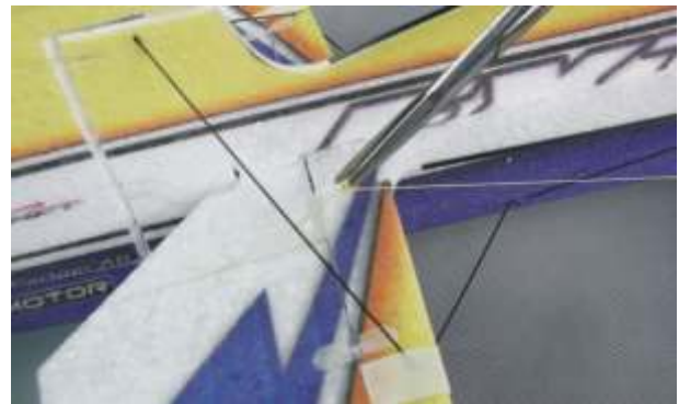
Make one of the thread end pass through the small hole on elevator, then tie a knot and glue it.
