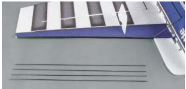
Cut off the 1mm carbon rod to 4 pcs of support rods for wing.
