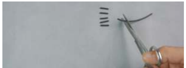
Cut off the shrink tubes to 6 pcs of 15mm.
