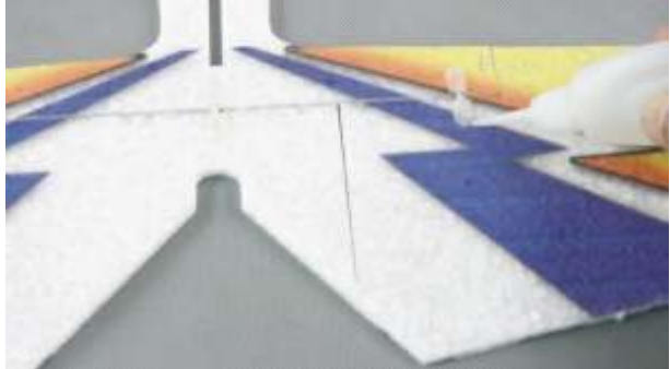
Insert the hinge to the pre-reserved seam and fix it with glue.
