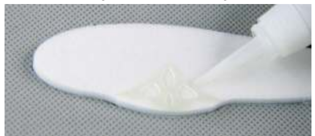
Install wheel cover reinforcement on wheel cover, and fix with glue.
