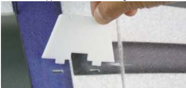
Install the support board of the wing first.
