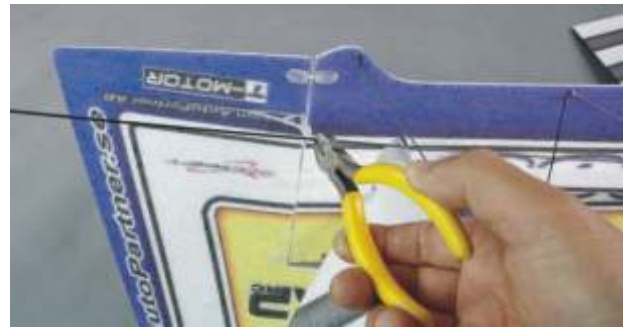
15. Installation of the pull-push rod.
