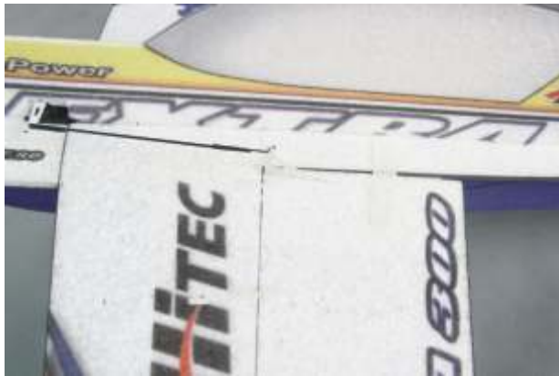
Fix the aileron for using adhesive tape, and then pass through the Z bend to the hole of control arm as picture shown.
