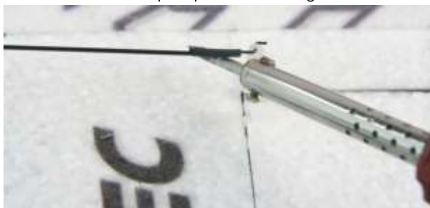
Fix the shrink tube with iron heating as picture shown.
