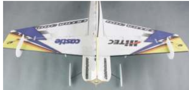
Install the wing fences to the left and right wing as picture shown.
