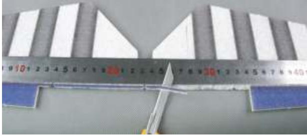
Cut off 45 bevel angle at the elevator.
