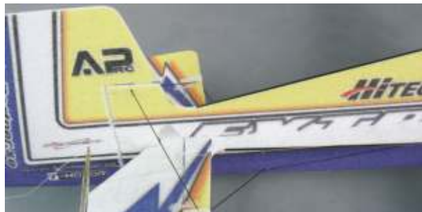
Cut off two pull-push threads. It will be 6-8cm longer than the distance from elevator servo to the elevator servo horn.
