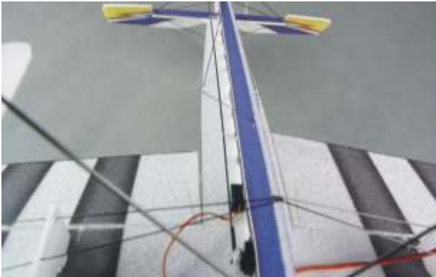
Make sure the pull-push rod is straight.
