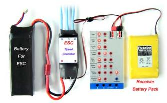
disconnect the BEC cable (trio wires) of the ESC from your receiver, then connect it to the program card at the top right corner position marked with "**BEC**".
