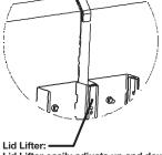
Lid Lifter easily adjusts up and down to provide a greater degree of flexibility when raising the TV out of the cabinet
