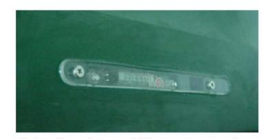
**Auto-dimming and IR remote receiver**(will be removed to front bezel next Ver.)
