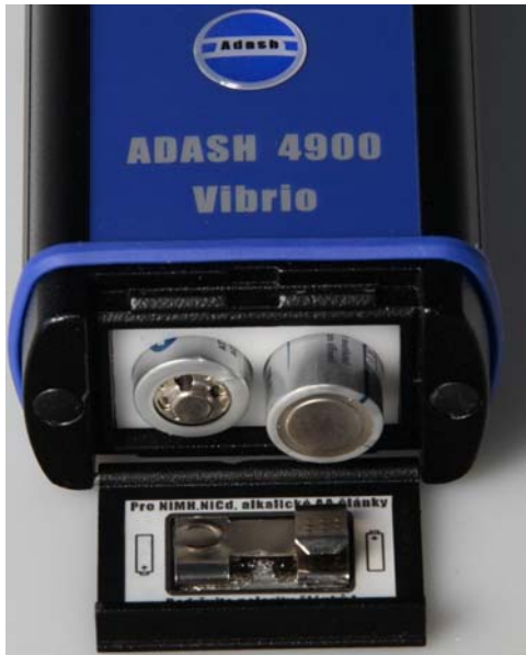
Fig. Placement of power batteries
