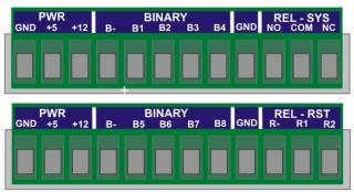
**PWR output** (A3716/3U only) is the source of +5V/1A and +12V/1A voltage outputs. All GND (grounds) clamps are shorted (connected together).
