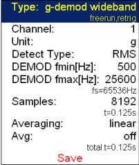
It is very similar to standard overall measurement. The signal is filtered in ( DEMOD fmin, DEMOD fmax) range and demodulated then.
