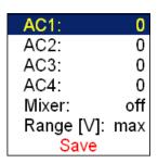
**AC1 – AC4** all channels can be mixed to one channel into wav file (like in music studio). The gain factor can be defined for each channel. When the zero is used, then this channel will not be used for mixing.
