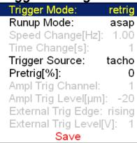
**Trigger Mode** This setting is used in Analyser and Octave Analysis modes.
