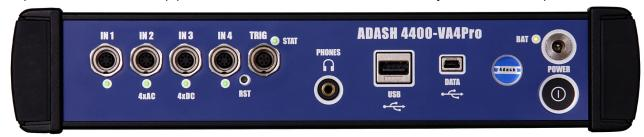
The input sockets labeled IN1, IN2, IN3, IN4 are used for AC or DC signals. The input socket labeled TRIG is used for trigger signals, usually tacho. All sockets have several pins. It enables to connect more signals to one socket (see wire diagrams).
