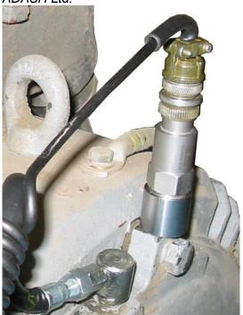
Sensor mounted near to lubrication point
