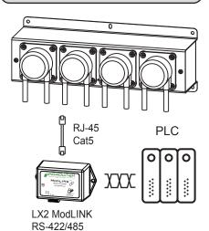
Agrowtek's digital variable speed peristaltic pumps are convenient and easy to implement on PLC systems with MODBUS RTU for advanced addressable communication. Use HX8 GrowNET™ hubs to network multiple devices to a PLC.
