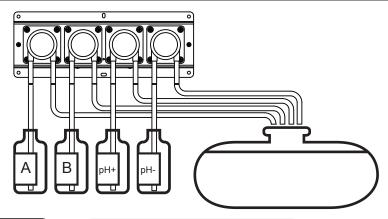
Concentrate Containers Any size or combination of solutions such as nutrients, pH buffers, etc.
