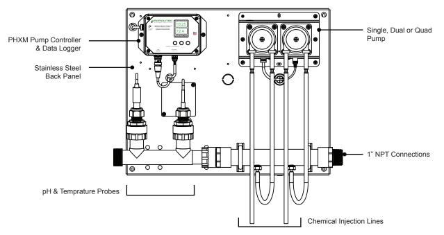
AgrowDose peristaltic pumps have legendary reliability, are self-priming, draw over 10ft of lift and pump into lines up to 25psi (up to 45psi with high-pressure check-valve kit.) Pumps feature easy-maintenance with no-tool, twist-off replaceable heads. Stainless steel back-panel makes installation as simple as hanging on a wall and connecting plumbing.
