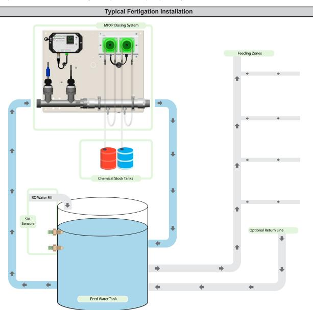
The dosing system is typically installed on a re-circulating loop for a master resevoir, or inline with a DWC bucket system pump. Continuous circulation and monitoring provides well regulated control of the water without the need to continuously check and dose manually.
