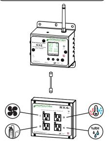
Connect the RX4i relay directly to Agrowtek's intelligent SXE climate sensors to create a basic environmental control system. Program outlets individually for temperature, humidity, or CO2 and cycle timer control. Uses the GrowNET ports and a cross-over cable to link the devices together.
