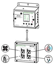
Combine a sensor and a RX4i or RD8i relay to form a powerful and economical basic control system. Configure standard control functions on the sensor to operate a relay module without a controller. Log data to the sensor's internal memory or add the WiFi module for browser access or web portal logging, email alerts, and more.
