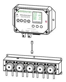
Combine a SXHM Hydro sensor and AgrowDose pump to form a powerful and economical automatic nutrient and pH (+ORP) dosing system. Configure basic dosing functions on the sensor screen to operate a dosing pumps without a controller. Log data to the internal memory or web portal, send email alerts and more.
