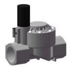
VX1 Water valve kit handles up to 20GPM @ 150psi and includes a 12Vdc wall power supply and adapter cable to operate the sensors and valve. UL Listed.
