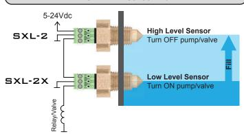
When liquid is below the high sensor (SXL-2, dry-on) its output provides power to the low sensor (SXL-2X, dry-on latching.) When liquid falls below low sensor, its output latches on. The low sensor's output is used to power a device (such as a control relay for a pump or valve) until it is reset by the high sensor's output turning off.
