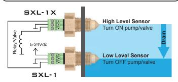
When liquid is above the low sensor (SXL-1, wet-on) its output provides power to the high sensor (SXL-1X, wet-on latching.) When liquid rises above the high sensor, its output latches on. The high sensor's output is used to power a device (such as a control relay for a pump or valve) until it is reset by the low sensor's output turning off.
