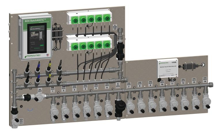
Expansion of a BatchMatic™ BDX fertigation system is as simple as mounting and connecting the manifolds, connecting the RJ-45 data cable, and plugging in the power supply. BDX systems can be expanded from 6 to 14 zones with the VXP8 expansion panel.
