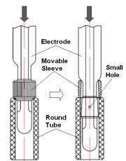
To loosen the movable sleeve, push up the movable sleeve. If it is too tight to push up, please refer to the right picture: insert the probe into the orange round tube (the accessory comes with the probe), and press down the electrode with force, then the movable sleeve will be loose. And then screw counter-clockwise to loosen the movable sleeve or clockwise to tighten it.
