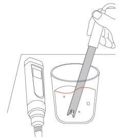
5.1.4 If necessary, turn on the Auto-Hold function (refer to Section 8.3.3), the reading will be automatically locked when it's stable for more than 10 seconds. Short press (CAL) to cancel the Auto-Hold and keep measuring.
