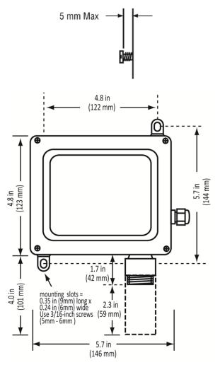
Figure 2. MGS-350 IP66 Housing (with Splash Guard)
