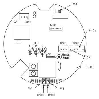
Figure 12. Adjusting Alarm Relays on the Mother Board
