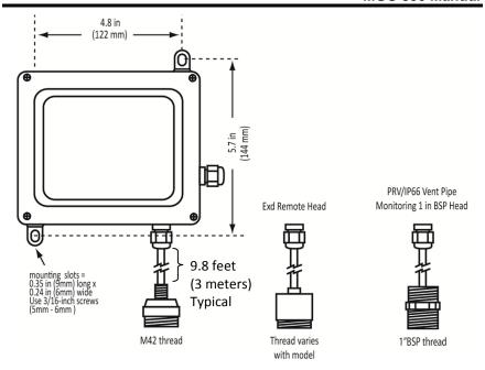
Figure 6. IP66 Housing with Remote Sensor Head
