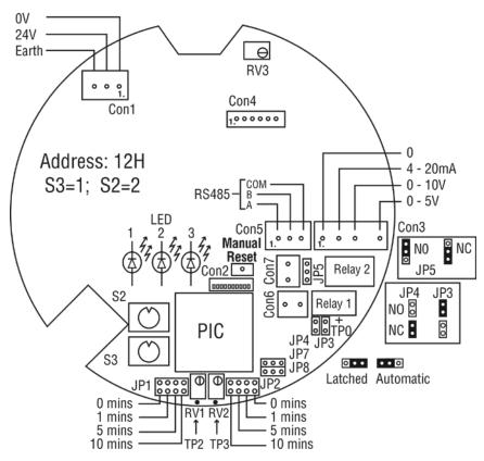
Figure 7. MGS-350 Connections and Key Components
