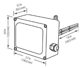
Figure 4. IP66 Duct Mount Housing
