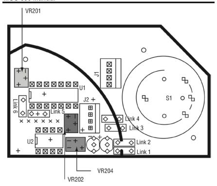
Figure 15. EC Sensor Board
