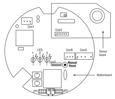
Figure 11. Example Sensor Board and Motherboard
