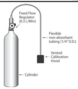
Figure 8. Gas Cylinder and Test Hardware
