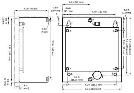
Figure 1. MGS-350 Standard Housing
