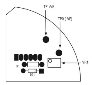
Figure 10. Example Pre-calibrated Sensor Board
