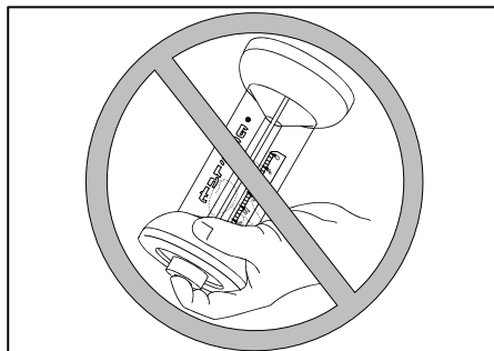
Figure 1d. NEVER vent FYRITE in the inverted position, which will cause fluid to spill.
