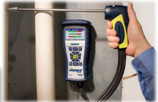
Intuitive setup screens and color graphics are sharp and clear in any setting. Unique hotspot finder detects optimal measurement site.
